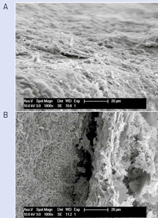
**Figure 1:** SEM of implants retrieved after 52 weeks: SurfLink® Dental treated implant surface showing cells attaching and spreading (A), control denuded implant surface (B), and pre-implantation pristine implant surface (C).
