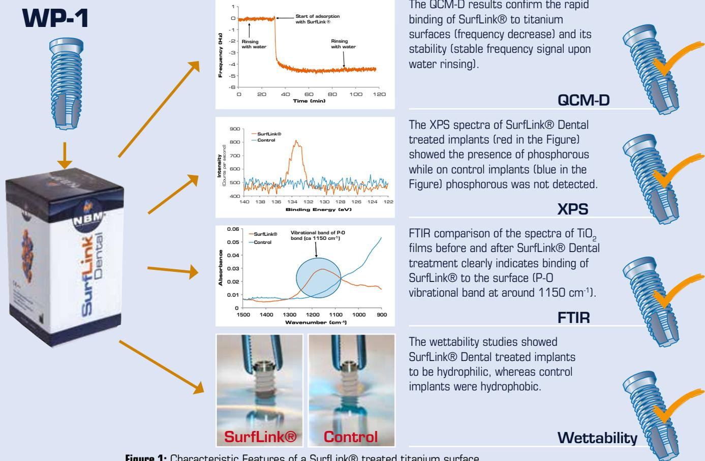
**Figure 1:** Characteristic Features of a SurfLink® treated titanium surface.
